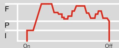
F = Full load; P = Partial load; I = Ignition load
