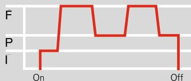
modulating (gas operation) with external load controller
