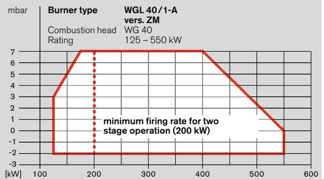
Capacity graphs in accordance with EN 676. The ratings are based on an installation altitude of 0 m. An altitude-based reduction in capacity of approx. 1 % per 100 m above sea level should be taken into consideration.
